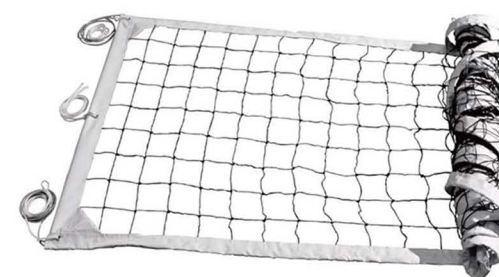
VB-006 PE Volleyball Net 1. Size: 9.5m x 1m 2. Net: 2.5mm PE 10cm twisted knotted net 3. Top: 0.55mm white PVC band x 2" 4. Sides 0.55mm white PVC band x 2.5" 5. Bottom: 0.55mm white PVC band x 2" 6. With a 5mm steel cable on top and bottom 7. Equipped with 2 dia 11mm solid fibreglass poles 8. Packing: 1 set in PE bag, 4 sets in carton
