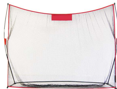
GN-001 Golf Hitting Net 1. Size: 10*7*3' 2. Pole Frame: Φ12.7mm fiberglass & Φ25*1.0mm steel tube 3. Net: polyester 7 ply 1.5" net with 420D sleeve
