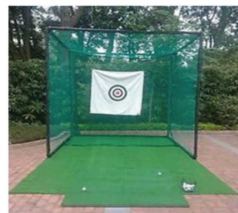
GN-011 Golf Cage Net 1. Size: 3 x 3 x 3m 2. Net: 1.5mm PE twisted knotted net 3. Frame: 28.6mm dia x 1.0mm thick 4. Target: 14oz white canvas & shooting print 5. Packing: Net, target, frame in 3 bag, 1 set in carton
